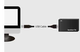
6. Connect the USB cable. (Power will be drawn from the USB port and provide power to the hard drive)
