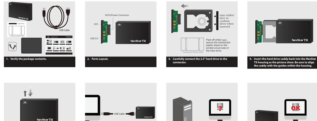
5. Secure the caddy to the housing using the screws provided.
