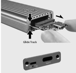
3. Remove the plate and slide out the Printed Circuit Board (PCB) by the side edge.
