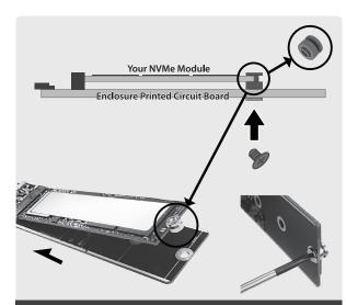
5. Use the screw nut provided, insert into the semi-circular notch of your M.2 module, press down the M.2 module and secure the M.2 screw nut using the screw from the underside. NOTE the orientation of the screw nut.
