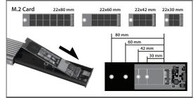
4. Your M.2 NVMe module may come in different lengths. Connect your M.2 NVMe module at an angle into the M.2 interface on the Tray PCB. Your M.2 NVMe module is keyed and can only insert into the interface with the label facing up. If you are NOT using M.2 NVMe module, you are using the WRONG product. Please write to support@vantecusa.com for help.
